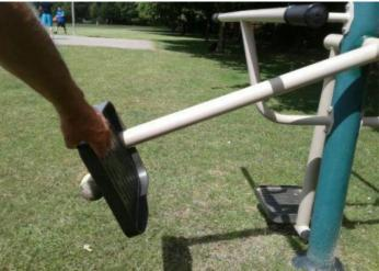
**Finding:** The swinging movement of the item exceeds the maximum 55 degrees from the vertical required by BS EN 16630
